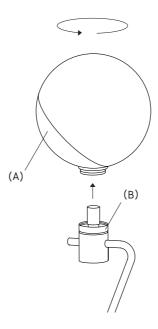
1. Unscrew the diffuser (A) while holding the metal ring (B).
