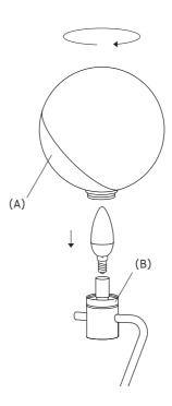
2. Insert the light bulb then gently mount the diffuser screwing it back to the metal ring.
