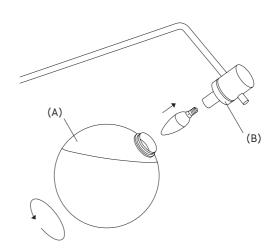
5. Insert the light bulb then gently mount the diffuser screwing it back to the metal ring.
