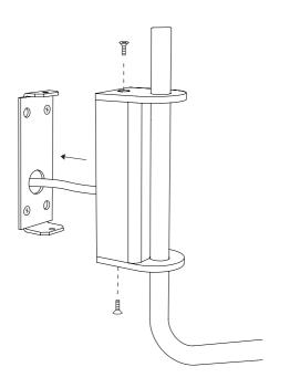
6. Attach the lamp body back to the wall mounting.
