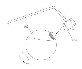
1. Unscrew the diffuser (A) while holding the metal ring (B).
