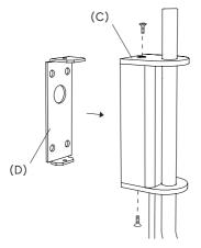
2. Remove the wall mounting (D) by unscrewing two screws from the lamp body (C).
