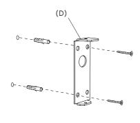
3. Mount the wall mounting to the wall with two appropriate screws and plugs. Always use correct screws and plugs for the mounting surface.
