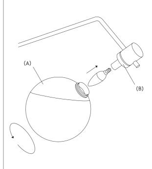
7. Insert the light bulb then gently mount the diffuser screwing it back to the metal ring.
