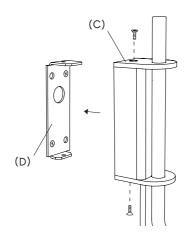
4. Attach the lamp body back to the wall mounting.
