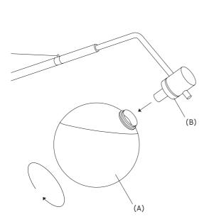
3. Unscrew the diffuser (A) while holding the metal ring (B).
