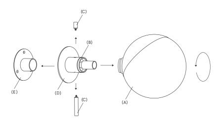
Unscrew the diffuser (A) while holding the metal ring (B). Unscrew the two screws (C) to dettach the mounting plate (E) from the lamp body (D).
