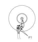
4. Connect the electrical cable with the terminal strip (F).
