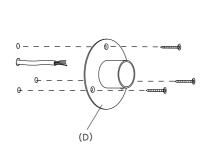
3. Mount the mounting plate to the wall with three appropriate screws and plugs for the mounting surface.
