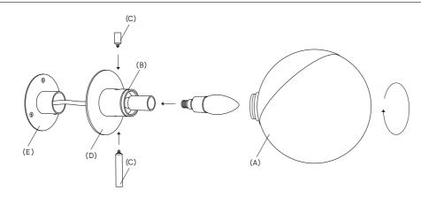
Attach the lamp body by screwing back two screws. Insert the light bulb then gently mount the diffuser screwing it back to the metal ring.
