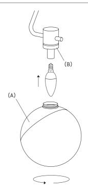
Insert the light bulb then gently mount the diffuser screwing it back to the metal ring.
