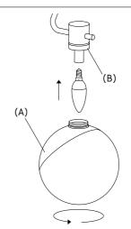
5. Insert the light bulb then gently mount the diffuser screwing it back to the metal ring.
