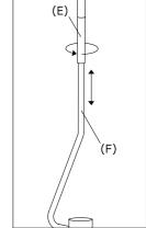
To adjust the lamp length, loosen the shaft (E) and pull the lamp body (F) to desired length.
