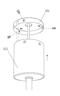
Attach the lamp body back to the wall mounting while making sure that ceiling mounting is covering the hole on the lamp housing.
