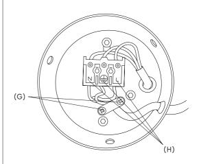
Unfasten the two screws (G) from the back of the lamp housing. Press N, ⊕, L tabs (H) on terminal strip to pull the cable out.
