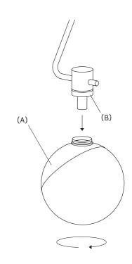
1. Unscrew the diffuser (A) while holding the metal ring (B).
