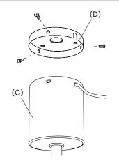
2. Remove the Ceiling mounting (D) by unscrewing three screws from the lamp body (C).
