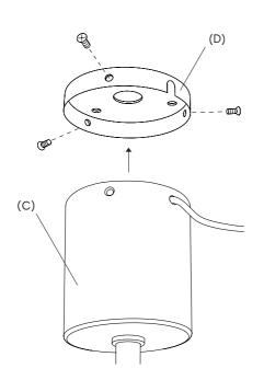
2. Remove the Ceiling mounting (D) by unscrewing three screws from the lamp body (C).
