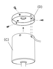
4. Attach the lamp body back to the wall mounting. Align the cable on the lamp body with groove on the ceiling mounting.
