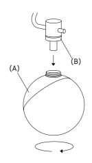
1. Unscrew the diffuser (A) while holding the metal ring (B).
