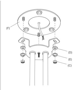
Attach the chandelier to the ceiling mounting (F). Place back the washer (D), spring washer (E), and tighten everything with the nut (C).
