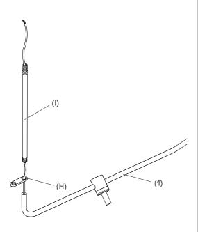
Assemble the first arm (1) and pull the cable through the spacer (H) and the vertical pipe (I). Screw the vertical pipe (I) into the arm (1) until it is hand tight. Do the same for the second arm.
