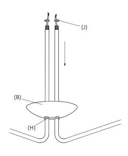
4. Unscrew the round threaded shims (J), slide the ceiling rose mask (B) to the spacer (H), and screw back hand tight the round threaded shims (J).
