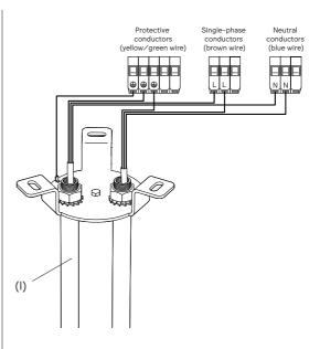
Connect the electrical cables from the vertical pipes (I) to the terminal strips. One terminal strip should hold all the protective conductors (yellow/green wires ⊕), the second one all the single-phase conductors (brown wires L) and the third one all the neutral conductors (blue wires N).
