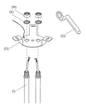
Tighten the bottom holder (G) to the pipes (I) by placing the tooth washers (K) and screwing nuts (M) with the provided tool (O).
