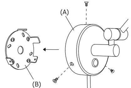
3. Attach the lamp body back to the wall mounting.
