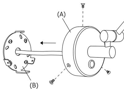
5. Attach the lamp body back to the wall mounting.
