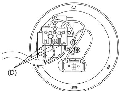
4. Connect the electrical cord with the terminal strip.
