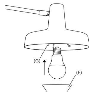
6. To insert the light bulb, release the undershade (F) by pressing three undershade brackets (G) inwards.
