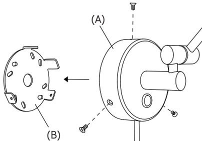
1. Remove the wall mounting (B) by unscrewing three screws from the lamp body (A).
