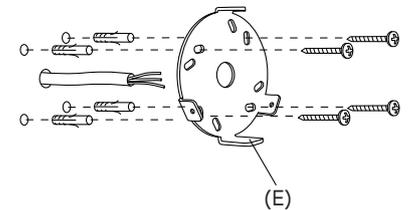
3. Position the wall mounting making sure the metal handle (E) is covering the hole on the lamp body. Mount it with four appropriate screws and plugs. Always use correct screws and plugs for the mounting surface.
