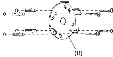
2. Mount the wall mounting to the wall with four appropriate screws and plugs. Always use correct screws and plugs for the mounting surface.
