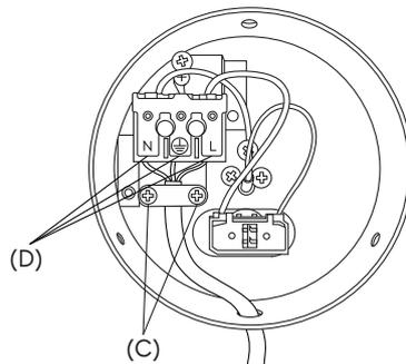
2. Unscrew the two screws (C) from the back of the lamp housing. Press N, ⊕, L tabs (D) on terminal strip to pull the cord out.
