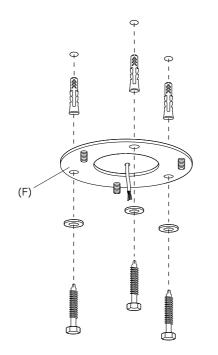
8. Mount the ceiling mounting to the ceiling with three appropriate screws and plugs. Always use correct screws and plugs for the mounting surface.
