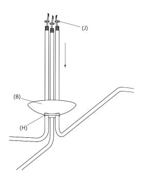
4. Unscrew the round threaded shims (J), slide the ceiling rose mask (B) to the spacer (H), and screw back hand tight the round threaded shims (J).
