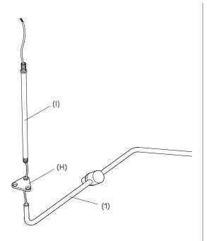
Assemble the first arm (1) and pull the cable through the spacer (H) and the vertical pipe (I). Screw the vertical pipe (I) into the arm (1) until it is hand tight. Do the same for the arms (2) and (3).
