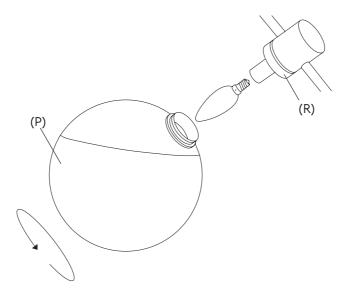
12. Take off the protective foil from the pipes. Insert the light bulb then gently mount the diffusers (P) screwing them while holding the metal ring (R).
