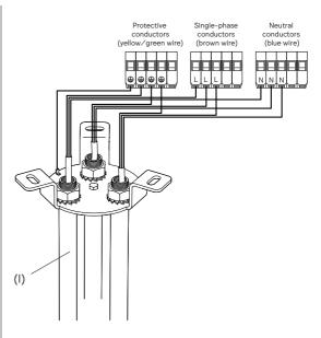
7. Connect the electrical cables from the vertical pipes (I) to the terminal strips. One terminal strip should hold all the protective conductors (yellow/green wires ⊕), the second one all the single-phase conductors (brown wires L) and the third one all the neutral conductors (blue wires N).
