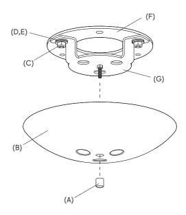
Unscrew the cylinder nut (A) under the ceiling rose (B). Unscrew the nuts (C), remove them together with washers (D) and spring washers (E), separate the bottom holder (G) from the ceiling mounting (F).
