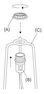
2. Pull the lampholder through the lamp frame (C). Tighten it by screwing back the top ring.
