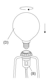
3. Screw the glass diffuser (D) onto the lampholder.
