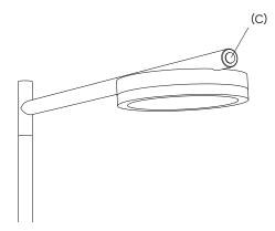
2. To turn on the lamp, tap the switch button (C) located on the horizontal arm. Hold the switch button to adjust light intensity.
