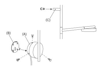
Remove the wall mounting (B) by unscrewing three screws from the lamp body (A). Also, unscrew the upper wall mounting (C) by unscrewing allen screw with 2mm allen key.
