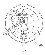
4. Unscrew the two screws (F) from the back of the lamp housing. Press N,  $\textcircled{\oplus}$ , L tabs (G) on terminal strip to pull the cord out.
