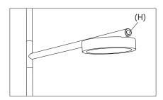
To turn on the lamp, tap the switch button (H) located on the horizontal arm. Hold the dimmer switch button to adjust light intensity.
