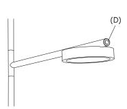
To turn on the lamp, tap the switch button (D) located on the horizontal arm. Hold the dimmer switch button to adjust light intensity.
