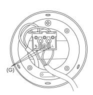
5. Connect the electrical cord with the terminal strip.
