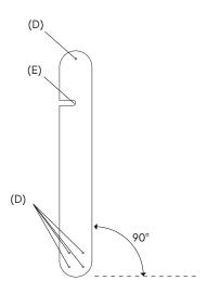
2. Place the cardboard template on the wall and mark plotted positions (D) so the position of rotating arm (E) is on desired height. Always pay attention that the cardboard plate is perpendicular to the floor.
